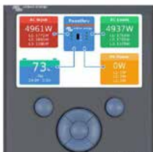
Color Control GX, showing a PV application
